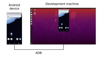
scrcpy = screen copy: remote display and touch input, does not require root
