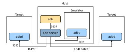
ADB is the link between development machine and Android device
